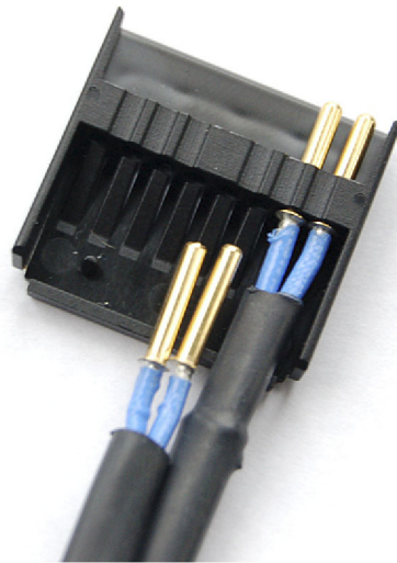
Figure 49: Inserting additional probe wires
